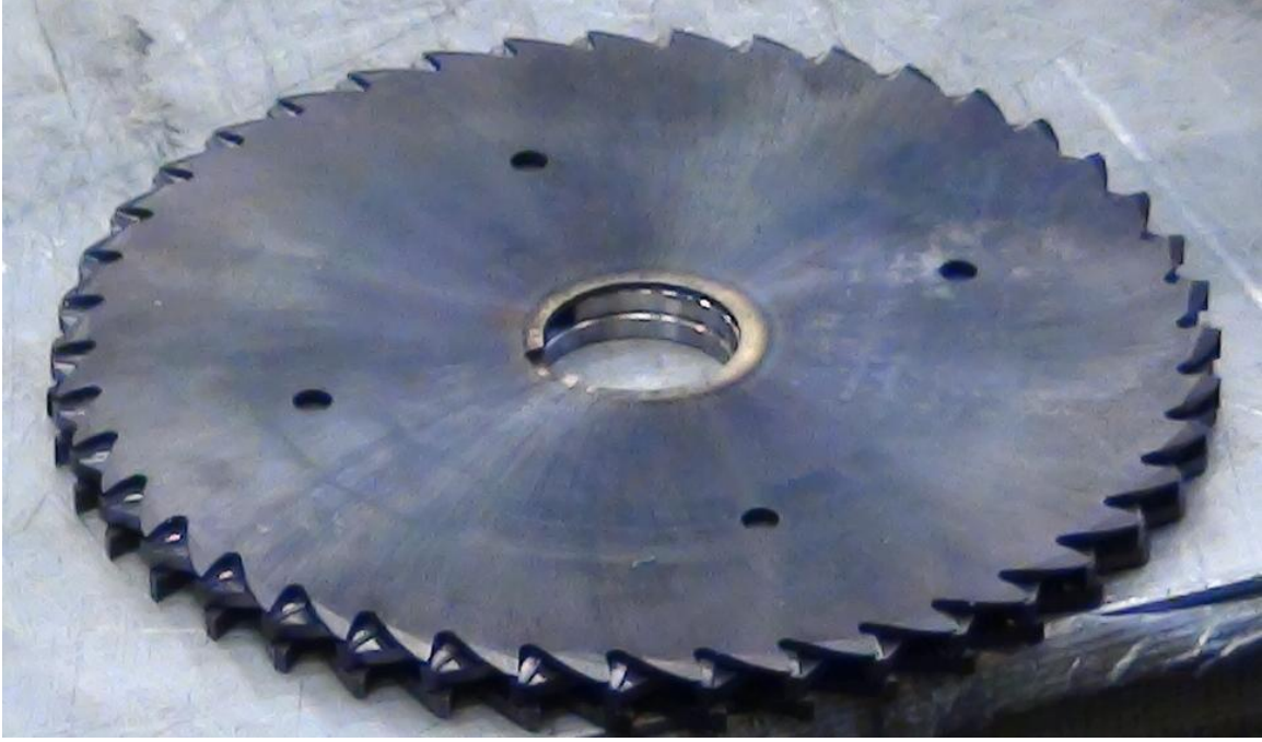
Figure 3.7. Blades used in machining the internal SC.
